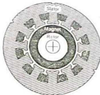
Fig 4.1 Arrangement of permanent magnet in the rotor
