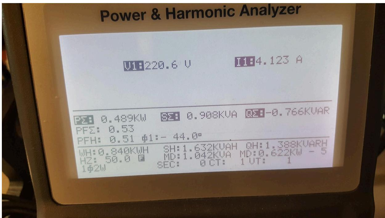
We have a large number of questions about Volts\*Amps not equalling power reported. The PCE830 shows that a large portion of the current is reactive.
