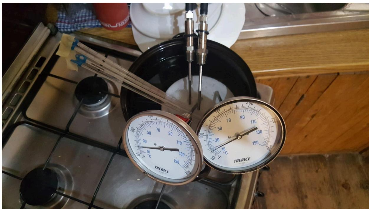
The water level dropped and the digital sensors were only partially submerged and ended up showing 96 at boiling. Had to add more water and let it get hot again. This allowed me to recapture a 90C data point. Last data point as temperatures come to steady level at boiling.
