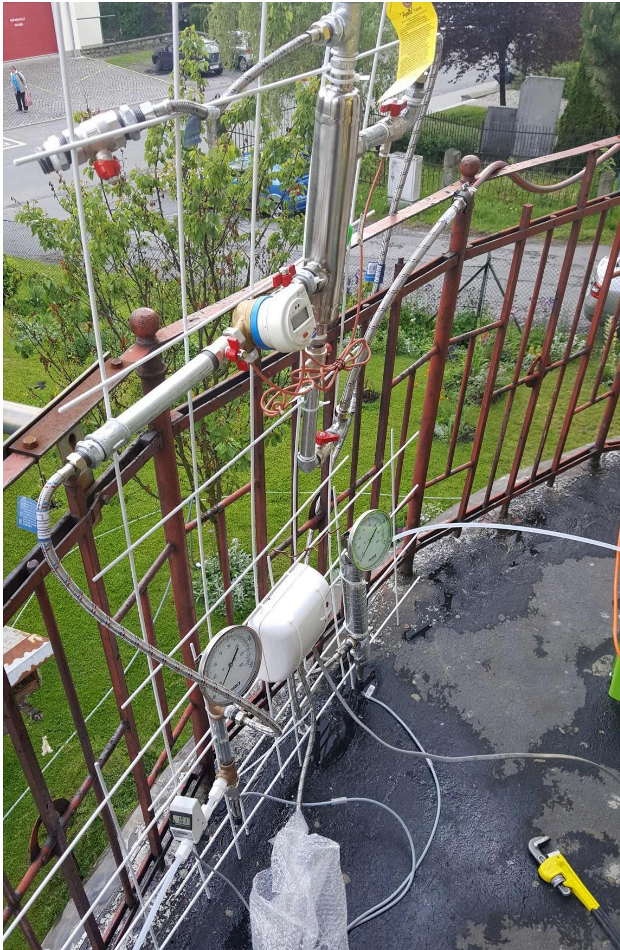
Plumbed in the heat exchanger instead of the water heater. Dealt with leaks. Measured over 6 L/min maxing out the flow meter. When we tuned it down the sensys meter was in close agreement to the Omega flow meter. Very encouraging. When the sensys says 0.060 m<sup>3</sup>/hr the Omega showed 1.01 L/min.
