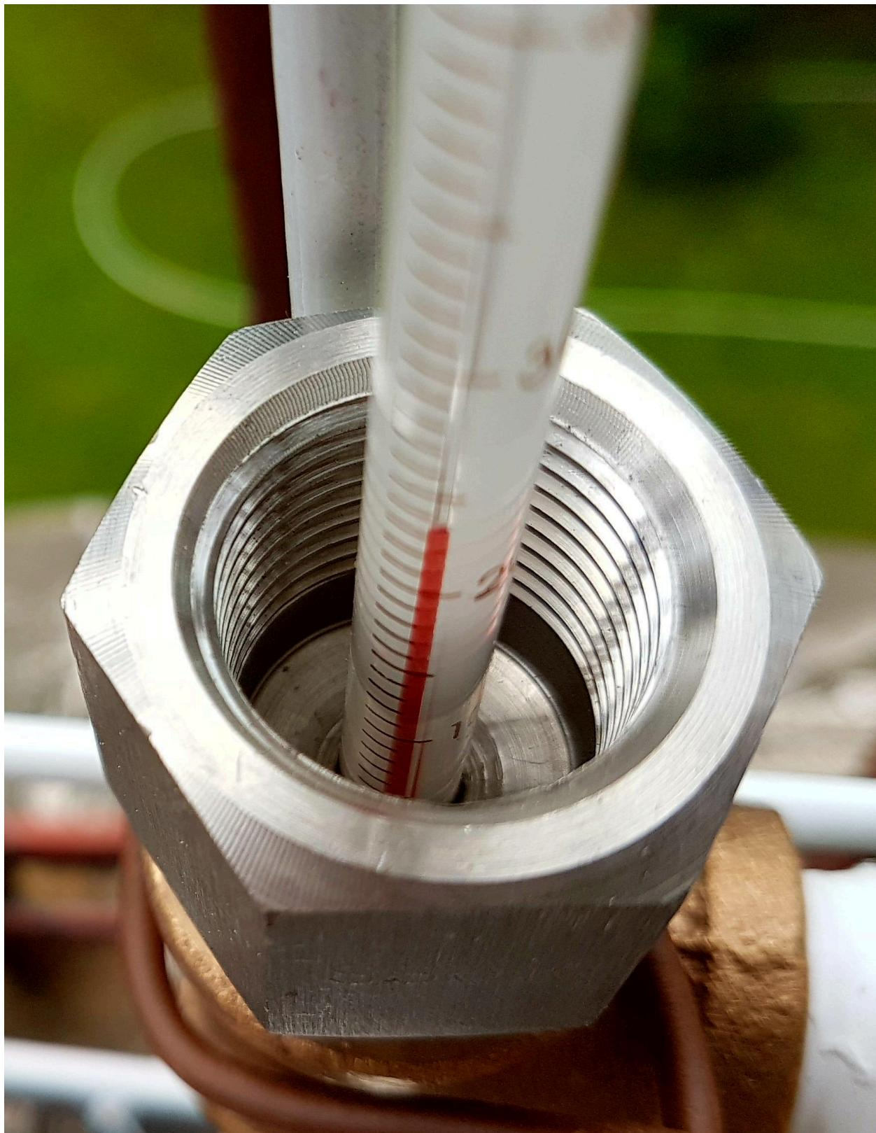
Depth of thermowell means that we will have to look into the thread to see below 20°C - down to 5°C is possible.
