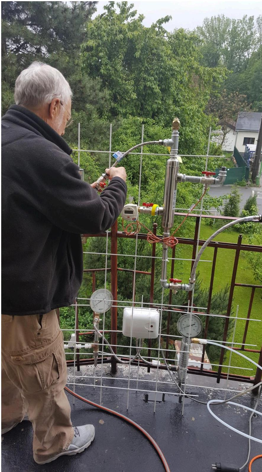
Meanwhile, Alan tested the hot side of the heat exchanger. No leaks in any hard joints. The water pressure here was adequate to pop the pressure relief valve, though. We have very little
