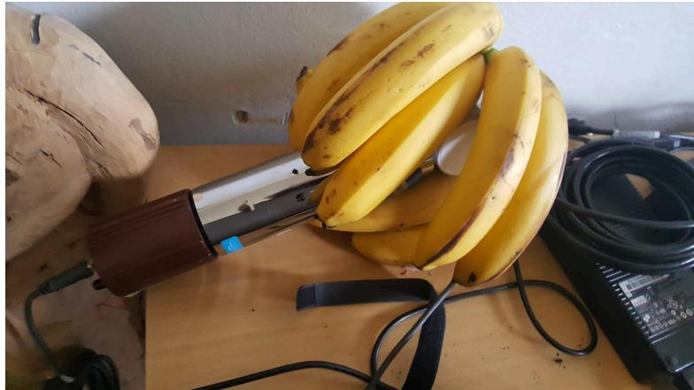
Shows the banana test with some K salt in addition. The detector failed to show a strong K peak. It was very modest 1.4 MeV peak.
