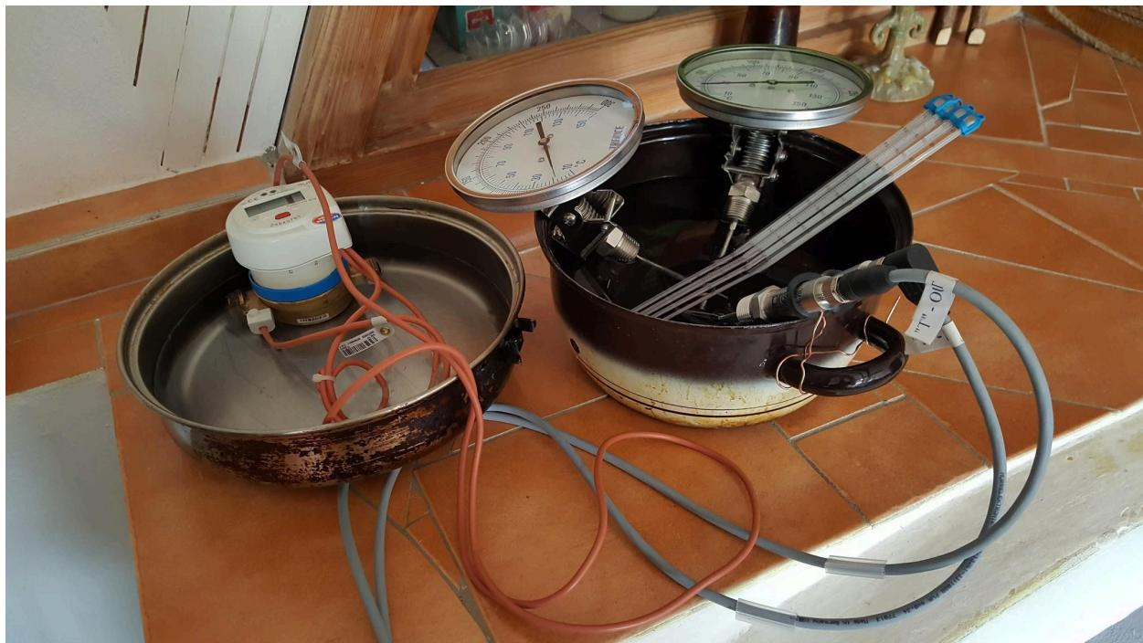
Sensys meter, too (since we have to submerge the entire unit we cannot boil it). The 2 temp sensors read only 0.018C apart
