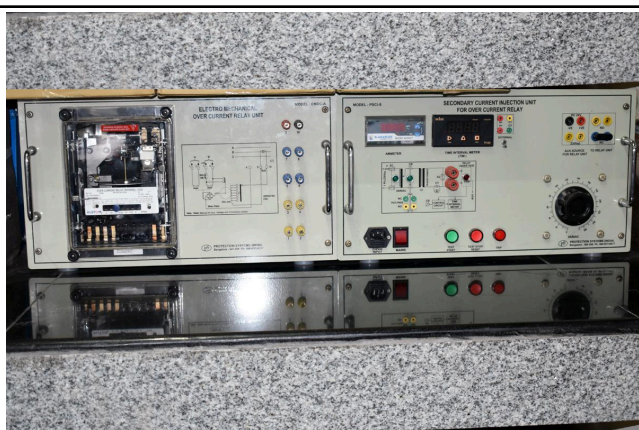
Electro Mechanical Over current Relay Unit
