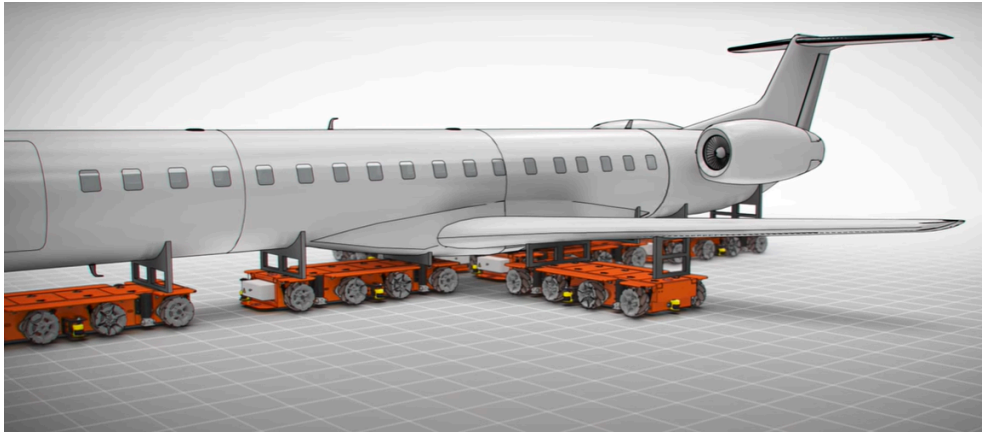
Figure 4: Kuka Transporting Mecanum Platform
