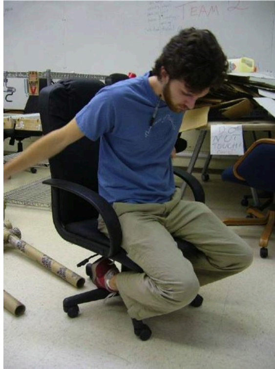
Figure 8: Testing different seating positions and reach using a chair. Notice the feet locked into position behind the rider. This gives the rider a high, upright posture. More detailed pictures of this test are located in Appendix 8.2
