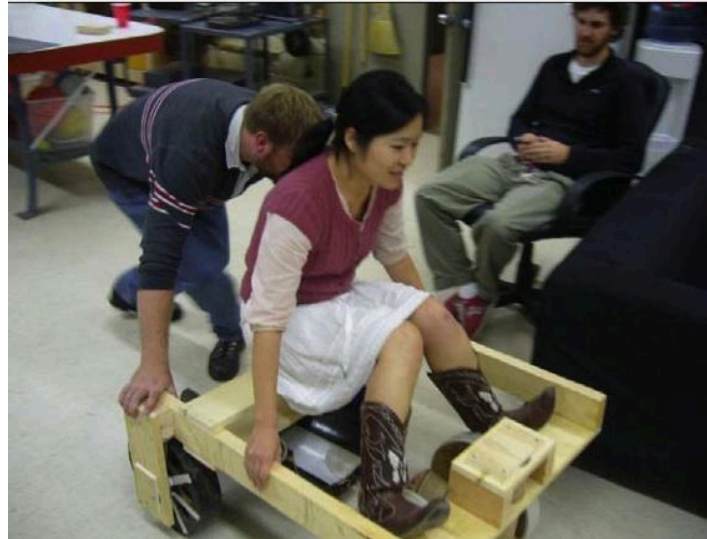
Figure 9: Function Prototype testing. Note that in this figure the caster is located in the front of the vehicle. Upon further testing, it was found that the caster worked best when located at the rear of the paper bicycle.
