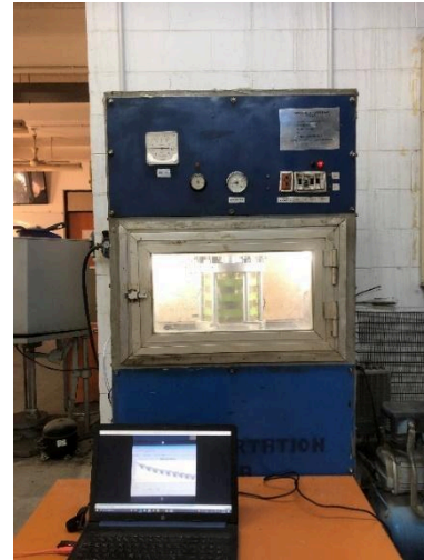
(b) Triaxial test under controlled temperature
