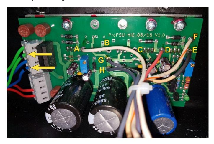
Carefully desolder the old wiring harness from the old power supply board.
