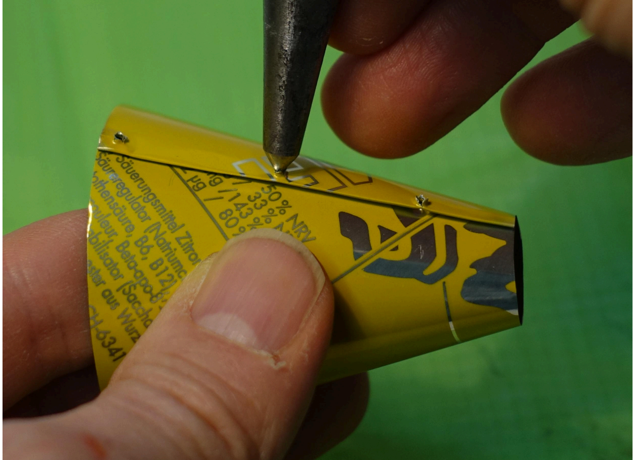
finishing the rivets
