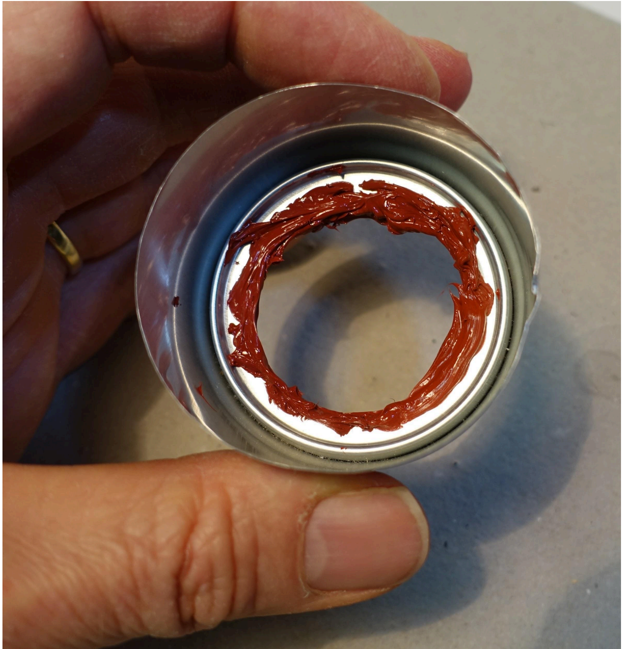
lid ready for final assembly, generously furnished with sealant
