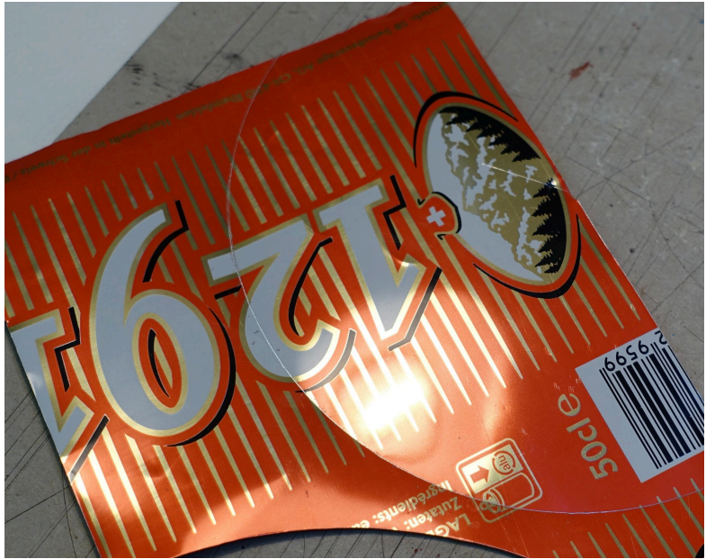
lower rim of the cone scored, ready for breaking the aluminum
