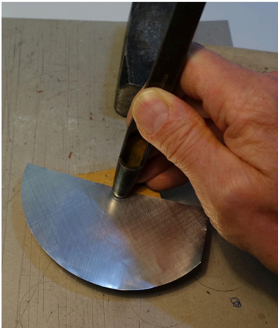
cutting the top of the cone with a hollow punch
