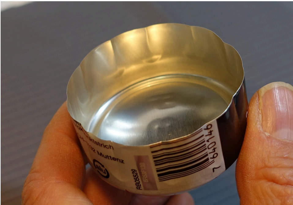
how the cup looks after the first round of indenting
