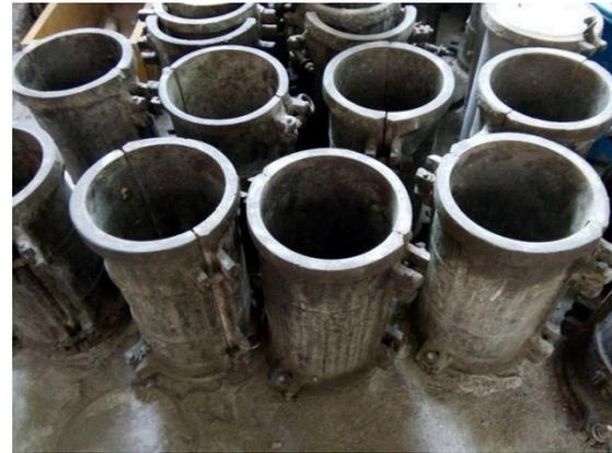
Gambar 1. Mould Silinder
