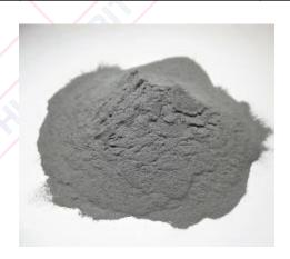
Electrolytic Iron Powder can be used in a wide range of applications including groundwater & soil remediation, powder magnetic cores, high-purity chemical manufacturing, pharmaceutical manufacturing, oxygen absorbers, paints/pigments, surface coating applications, additive manufacturing, metal injection molding, non-destructive testing, and more. It can also be used as a filler metal for plastics and epoxy's.
