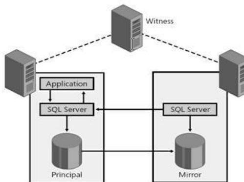
Gambar 1. Database Mirroring Architecture
