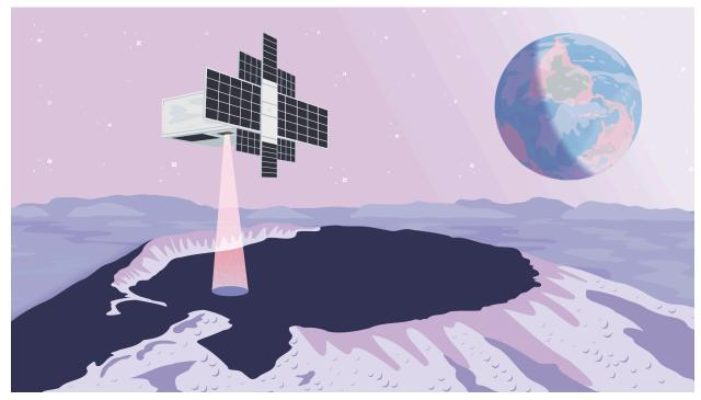
The Lunar Flashlight spacecraft shines a laser into a dark crater on the Moon, lighting up a circular area on the surface. Earth sits just beyond the horizon on the Moon's south pole, a perspective that makes Earth appear as if it has been flipped 180 degrees. Image credit: NASA/JPL-Caltech | + Expand image
