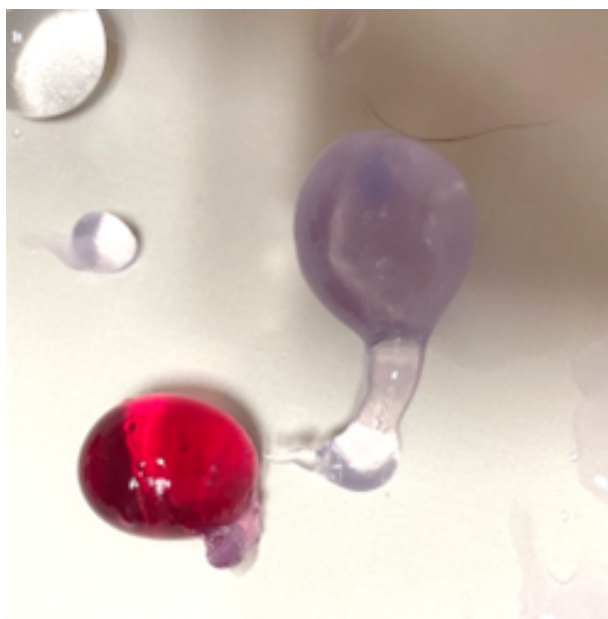
Figure 4. Beads can be produced in a wide variety of conformations. By changing the size of the dipping spoon, altering the dipping pattern, or using molds, a wide variety of shapes can be made.
