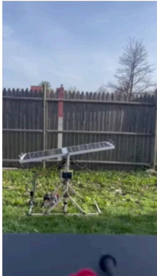
Figure 7.1.1: Solar panel starting position, showing the solar panel with the sun at its highest position ready to adjust the angle.
