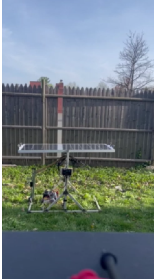
Figure 7.1.2: Solar panel adjusted position, showing the final position after letting the system run for a couple of minutes with the sun at the highest position.
