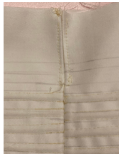
Fig 1.6. Center back finished with \frac{1}{2} inch, straight stitched seam, pressed.
