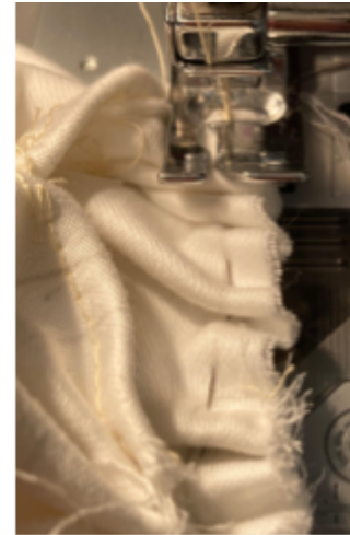
Fig 1.9. Machine sewing with 2mm straight stitch over bottom basting stitch, once \frac{1}{2} seam allowance is cut.
