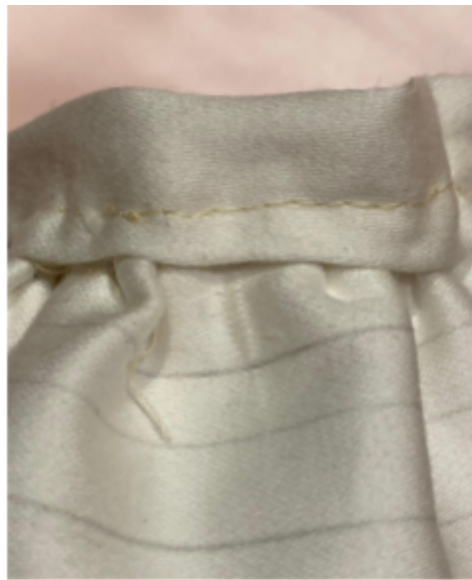
Fig 1.11. Finished exterior of waistband, finished with 2mm machine straight stitch.
