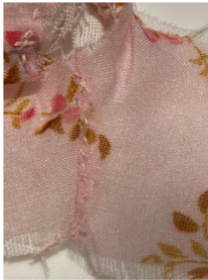
Fig 3.11. First topstitch made only from the self fabric.
