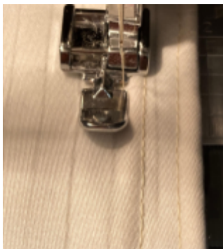
Fig. 1.2: Sewing in seam alongside second cording channel, with 3mm straight stitch.
