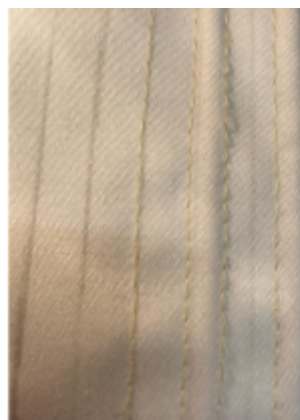
Fig. 1.3: First two initial lines of cording done, third channel seam sewn in.
