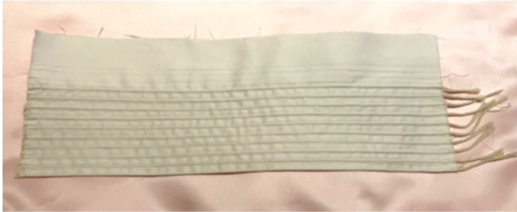
Fig. 1.4: cording is sewn up all channels using same technique and length of stitches, stops 3-5 inches from the top of the panel.
