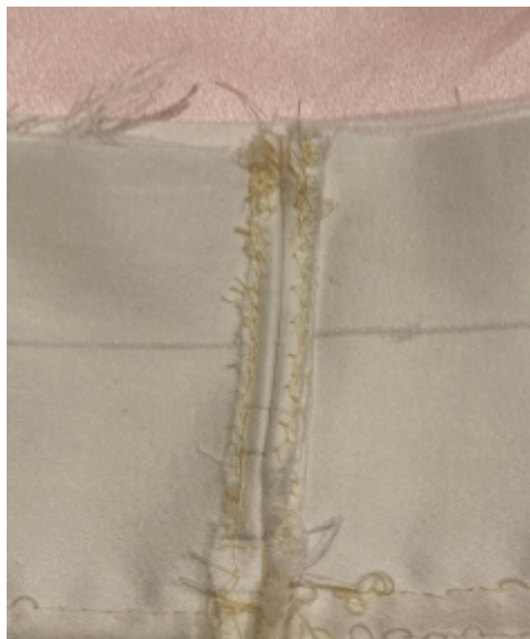
Fig 1.5.: Center back slit finished, with a 2mm zig zag stitch, pressed and turned over a \frac{1}{2} inch hem.
