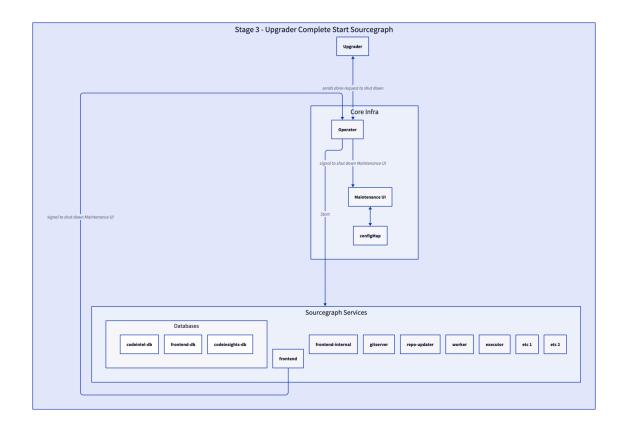
When the Upgrader is complete it signals the Operator it's ready to shutdown and Operator starts the other sourcegraph services. With this in place we can remove the migrator initContainer from the frontend deployment manifest.
