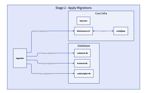
Here we see a new service Upgrader. This is essentially using migrator packages to run necessary operations from the upgrade and up command depending on what it necessary. This will operate very much in the same way as migrator except that it will also communicate its outputs to the maintenance UI to display to the admin the upgrades progress. Much of the logic necessary here can be reused from autoupgrade. Example
