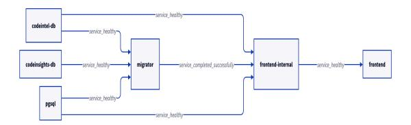
The diagram above depicts the startup pattern of a Docker-Compose deployment. Here we see that the databases are started first and that migrator must complete before other processes are started. Migrator is started with the up command. This ensures that the databases are in the expected state before frontend will start. In kubernetes deployments the same startup behavior is accomplished by running migrator as an initContainer of the sourcegraph-frontend deployment with the up command.
