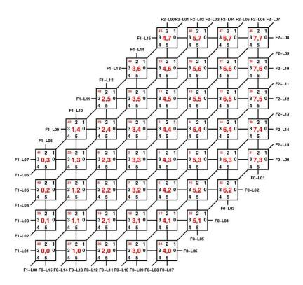
The FPGAs are connected internally to a subset of the border chips on the board as shown above; the links at the edges of the board are coded as F<fpga-id>-L<fpga-link-id>, so F1-L04 is FPGA 1, FPGA link id 4.
