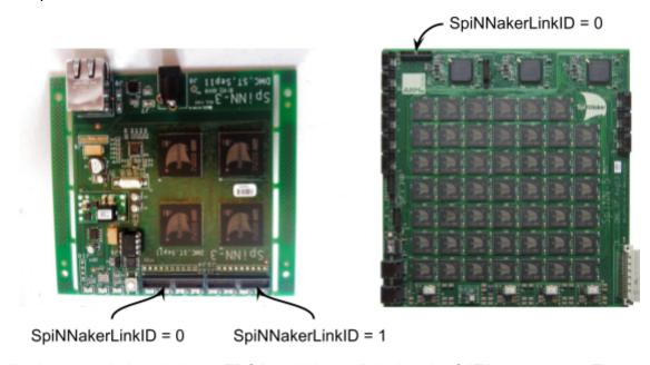
Additionally, the 48-node boards have FPGAs which are linked to the SATA connectors. These are shown below.
