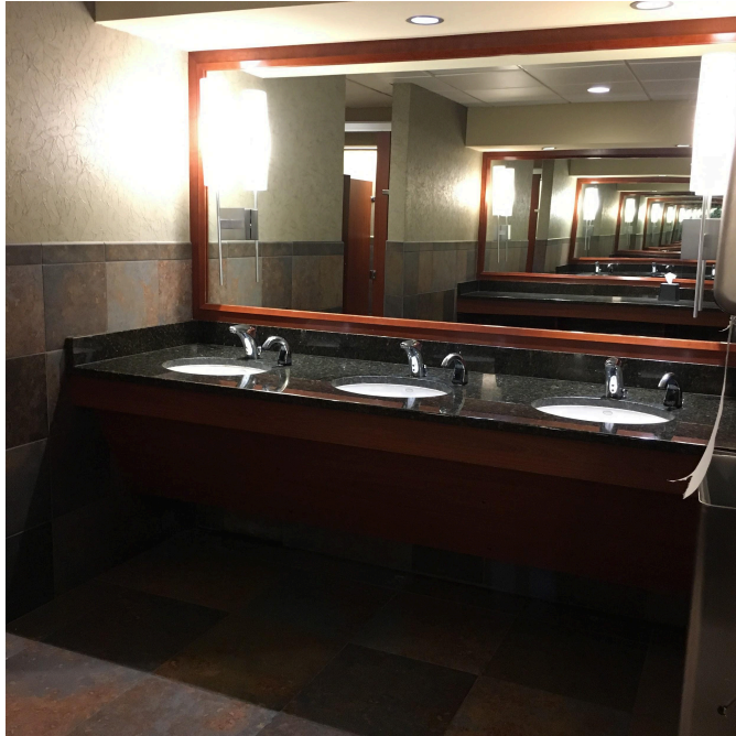
Image Description: Hyatt restroom interior with a sink area that allows for roll-under. The wall and floor are covered in mottled gray and rust slate tile.
