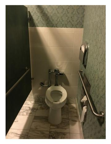
Image Description: Interior of the Hilton restroom accessible stall. The stall is long and narrow, with handrails on either side of the toilet. The toilet paper is installed below the handrail to the left of the toilet when one is seated, and the seat cover dispenser is above the same handrail about 40 inches from the ground.
