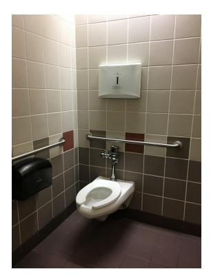
Image Description: Interior of Wisconsin Center accessible restroom stall, with handrails on the back wall above the toilet and on the side wall to the right when seated. A toilet paper dispenser is installed below the side wall handrail, and a seat cover dispenser is installed high on the wall above the back handrail.
