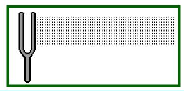
ALT TEXT: A tuning fork vibrates the particles of matter around it, creating a pressure wave of sound energy illustrated by a repeating pattern of particles that are compressed together, and particles that are spread out. The particles of matter carry the sound wave from left to right as they bump into one another,
