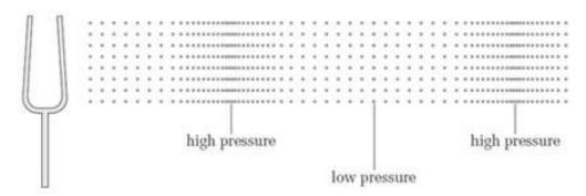
ALT TEXT: A sound generated by a tuning fork causes a periodic pattern of high and low pressure areas in a medium. Areas where particles are close together are labeled as "high pressure," and areas where particles are farther apart are labeled "low pressure." Source: Sound for Music Technology - The Open University
