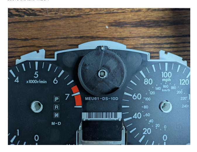
Next, attach the gauge assembly itself to the mount using a generous blob of hot glue underneath it. This is just to keep the gauge in place and properly aligned during assembly -
