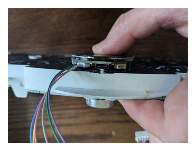
Next, plug in the speakers (if desired). Pull the harness up to the top of the cluster, so that none of it interferes with the turn signals etc and affix it to the white plastic on the cluster similar to this:
