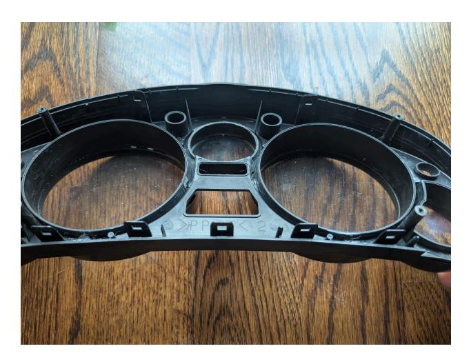
Next, install the bezel ring into the bezel. If you look at it from the side, you'll see that one portion is slightly thicker than the rest - that side faces the top of the cluster. I've found that friction will usually retain the trim ring well enough, but you can use a touch of hot glue to hold it in place if desired.
