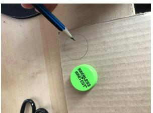
15. To make different-sized pinions, look around for circle-shaped objects of various sizes (bottlecaps, cups, etc). Trace these objects onto cardboard and cut them out.
