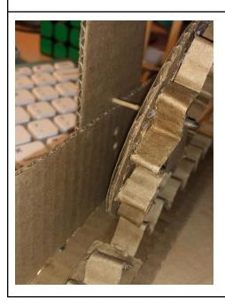
17. On the base plate, punch holes that align with the height of the center of each pinion.
