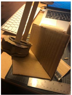
Glue the long edge of this piece to the long edge of the base plate (the edge opposite of the pinion)
