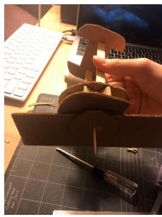
Put the pinion toothpick through the hole in the new piece of cardboard. Glue the circle to the other side.
