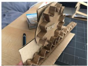
18. Attach pinion to the base plate using a toothpick (same as step 11).
