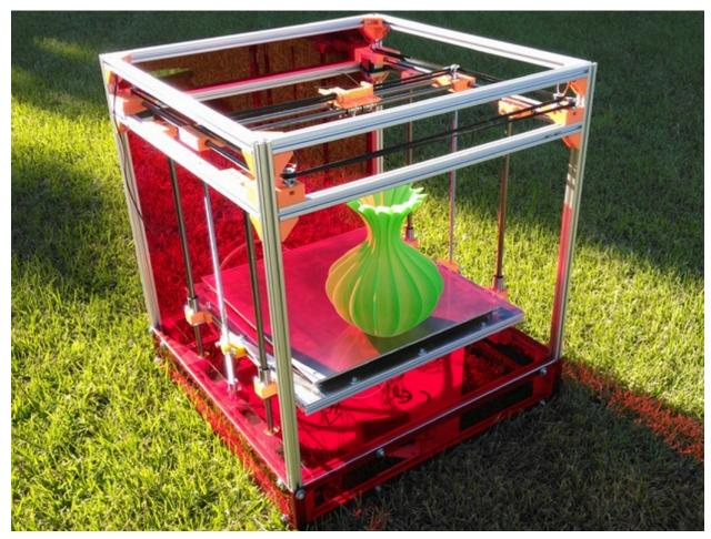
Use the Vulcanus concept of 2 threaded rods and 4 steel rods for the Z axis movement. Use One or Two motors to drive it to ensure precision and little time consumption for calibration?
