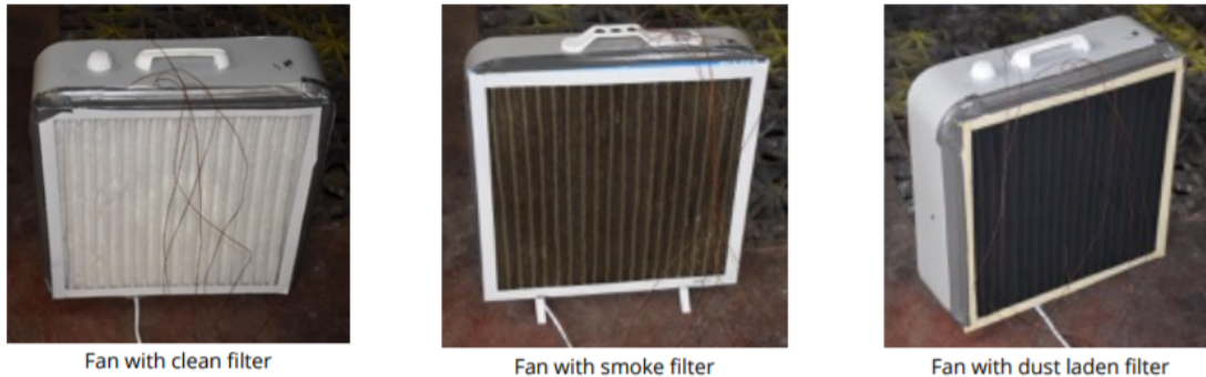
FIGURE 2. PICTURES OF TESTED BOX FANS WITH FILTERS AND THERMOCOUPLES ATTACHED.
