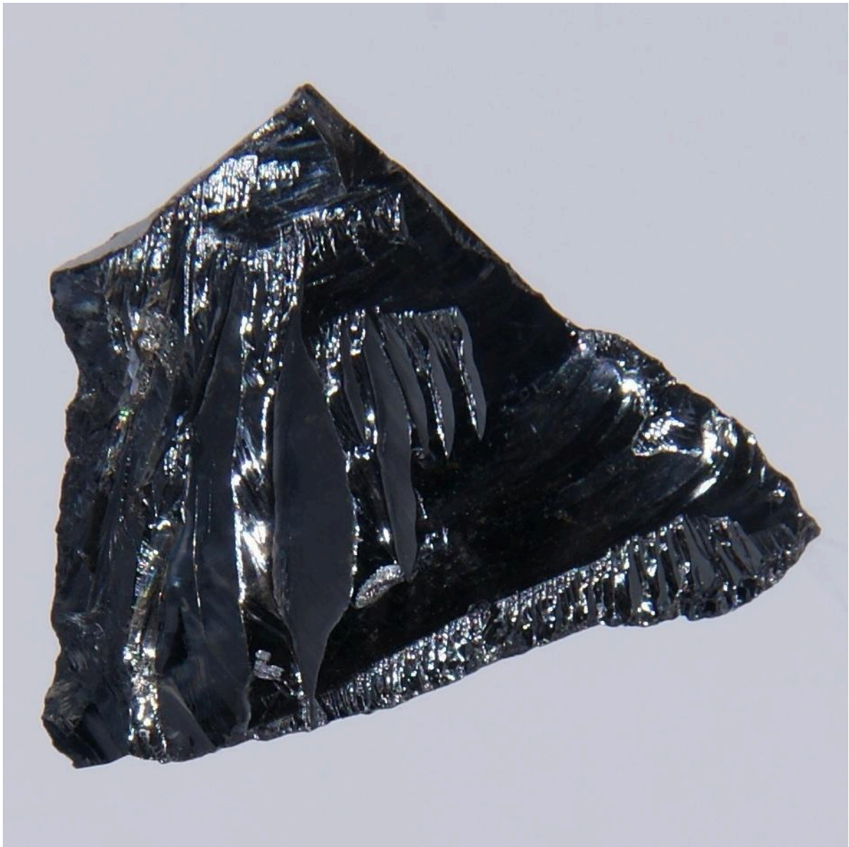
Silicon crystals are the most common semiconducting materials used in microelectronics. Image credit: images-of-elements.com
