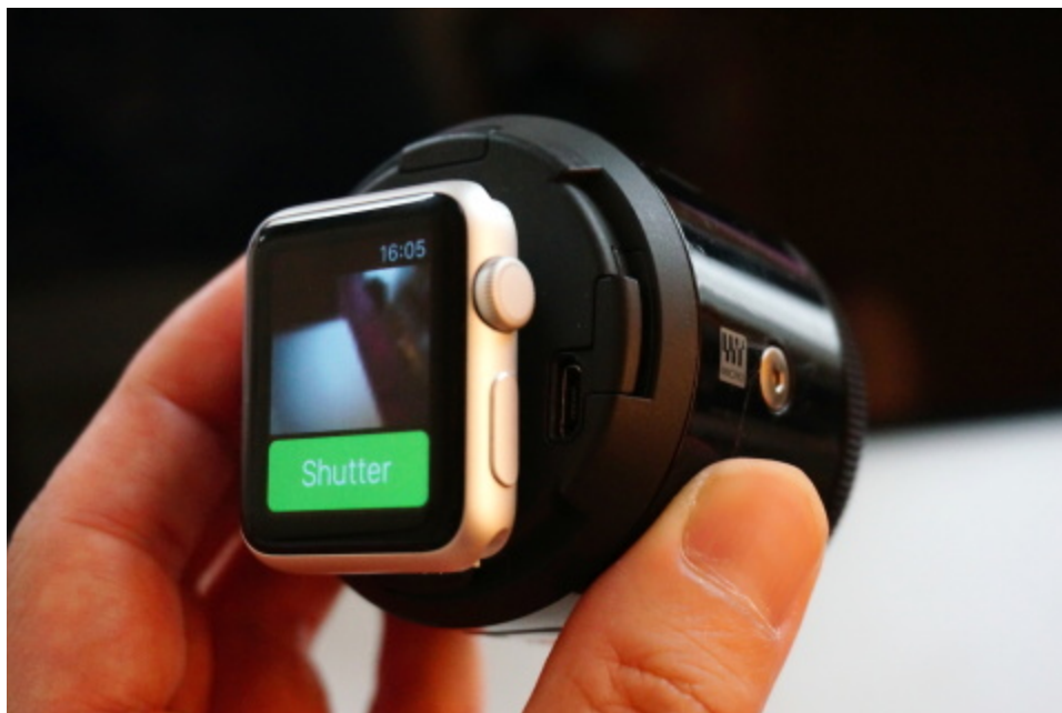
Olympus air hacked to work with the apple watch.
