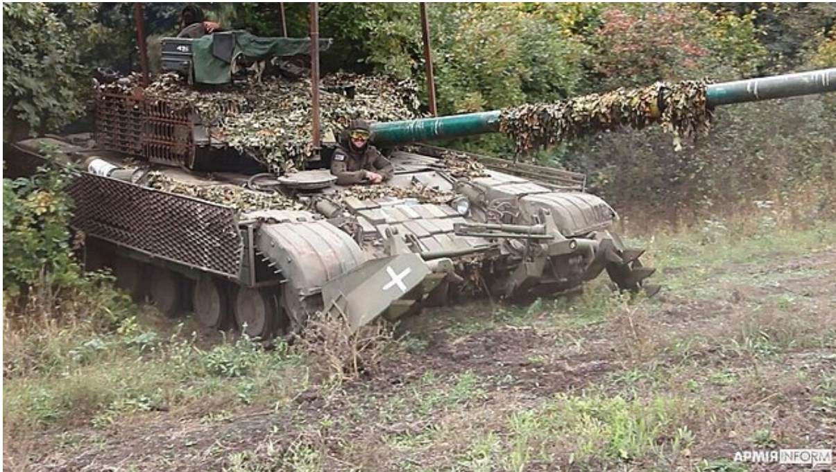
Figure 1 – Despite the proliferation of drones, tanks like this Ukrainian T-64 have opted for improvised protective cages rather than disappear from frontline combat altogether.
