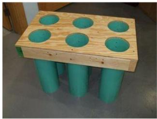
To use the tubes, you just need to flip it over and slide a bag on each tube. Roll it back upright and start shoveling to fill the bags. By design it will fill each bag to about 35lbs. Once you have filled all 6 tubes, pick it straight up and the sand will slide out of the tubes into the bags. Then you will have 6 perfectly filled sandbags.
