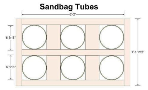
Once you have your frame, you can see how you will slide the tubes into each hole. You will need to put the 1-5/8 screws through the tube and into the sides where it touches the boards on all four sides. There should be two screws at each spot. First, take your drill and pre-drill the 8 holes on each tube; one at 1" from the top and one at 2.5" from the top every 90 degrees. Now put the tube in the frame and put screws in each hole. The easiest way is with a right angle drill.
