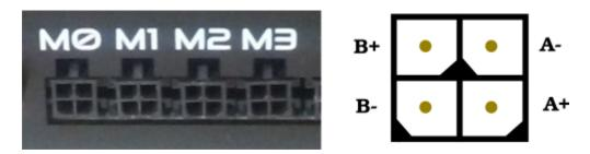
As you can see from the above picture you just need to get a connect to fit the onefinity controller (I bought the extension cable from Onefinity and cut the wire to connect it to my rotary motor so all I would have to do is splice the wires together and plug it into the controller.)
