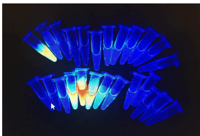
Image 1.4b: Gel Doc image of fractions following affinity chromatography of control using a GSH affinity column and an elution buffer containing 50mM of GSH. The first fluorescent tube shown in the above image is erroneous.
