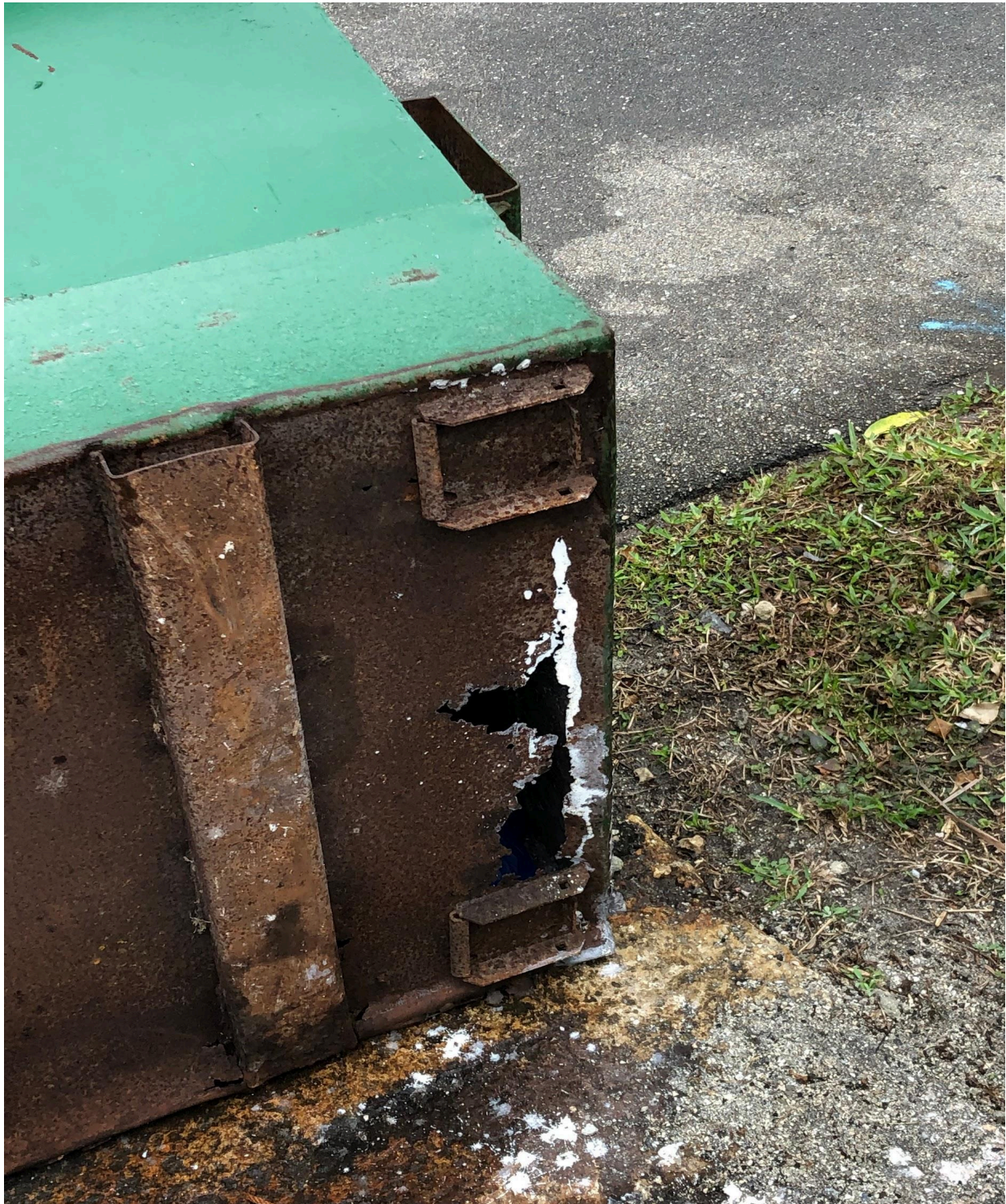
BEDFORD F- RUSTED OUT DUMPSTER. REPORTED IN BY A CV UNIT OWNER. REQUEST FOR REPLACEMENT WAS SENT TO WASTE PRO.
