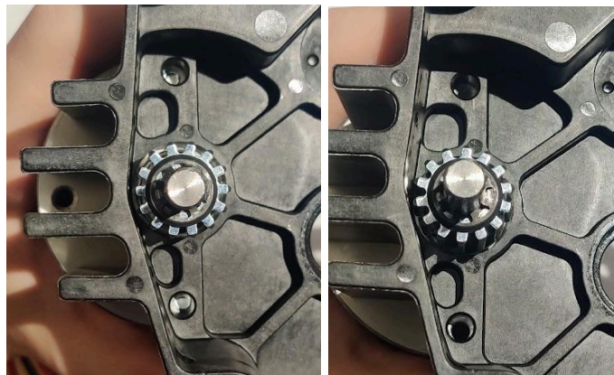
“Blocked” versus open mounting holes
