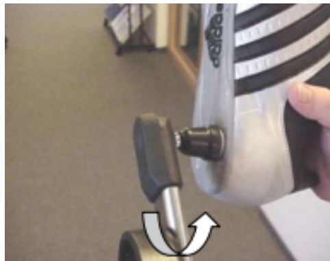
Figure 2 – Unscrewing the studs
