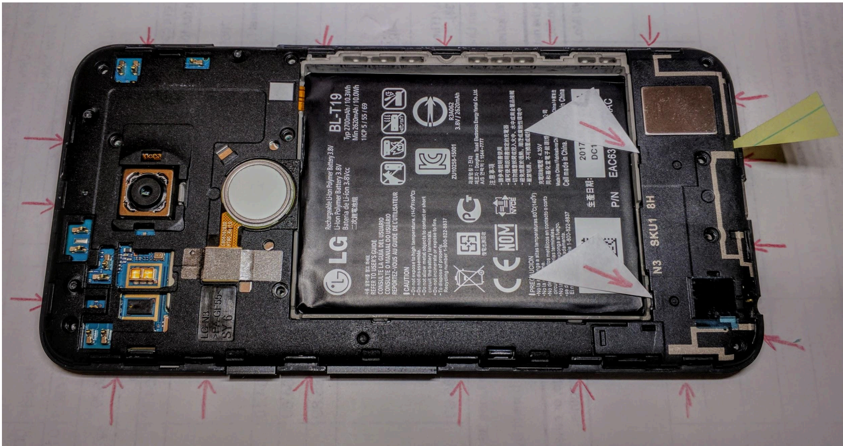
The location of the 20 tabs that hold the middle assembly in place. They're in the same places where the back cover tabs are . The yellow paper triangle is inserted where a pry would lift the middle assembly up in subsequent steps.
