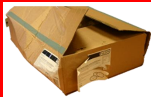
Broken or collapsed box Tape not applied
