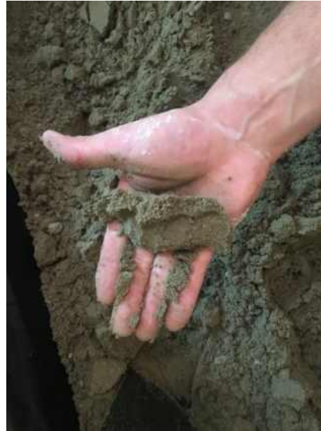
Fig.: Dry Pack Mortar Ready for Utilization
