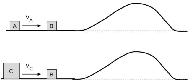
Block A, of mass M, is moving with a speed  $v_A$  to the right along a frictionless surface when it has a perfectly elastic collision with Block B (also of mass M). The speed  $v_A$  is the minimum speed that causes the mass B to slide over the frictionless bump. Now a different block C of mass 3M collides and sticks to block B. What is the minimum speed block C must travel (in terms of  $v_A$ ) in order for block B to slide over the frictionless bump?
