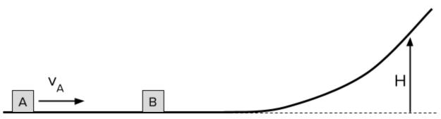
Block A, of mass M, is moving with a speed  $v_A$  to the right along a frictionless surface when it has a perfectly elastic collision with Block B (also of mass M) which makes block B slide up to a height H on the frictionless ramp. If the block A were again sent in with a speed  $v_A$ , but the collision were perfectly inelastic, what would be the new height block B will slide up the ramp?
