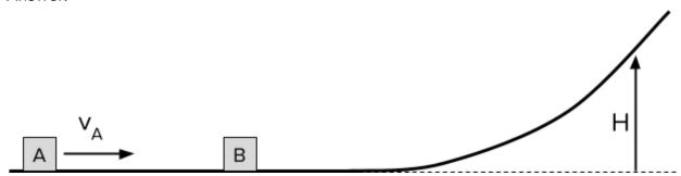
Block A, of mass M, is moving with a speed  $v_A$  to the right along a frictionless surface when it has a perfectly elastic collision with Block B (also of mass M) which makes block B slide up to a height H on the frictionless ramp. If the block A is sent in with a speed  $4v_A$ , causing another elastic collision, what will be the new height block B will slide up the ramp?
