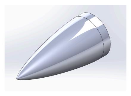
NOTE: Original Plan  $\rightarrow$  Wet Layups for the Nose Cone. Have since changed to prepregs (More on this after the "Profiles" Section))
