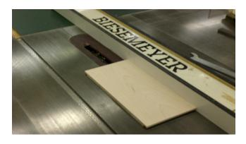
23. Next set up table saw or router table with a 3/8" blade or bit to notch for the fitted top.
