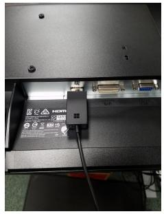
The other end of the USB extension cable plugs into the USB power adapter. This is necessary to get power to the Microsoft Display Adapter.
