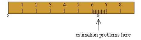
It is clear that our estimate was close, but the measurement still does not align with a mark. Not only that, but we are having trouble reading the marks now because they are so fine. Now we can estimate with a <a href="https://example.com/higher-precision">higher precision</a> that the measurement is 6.39, although you might say that it is 6.38 or even 6.40. Whatever it is, your best guess is 'correct' although it is not certain.
