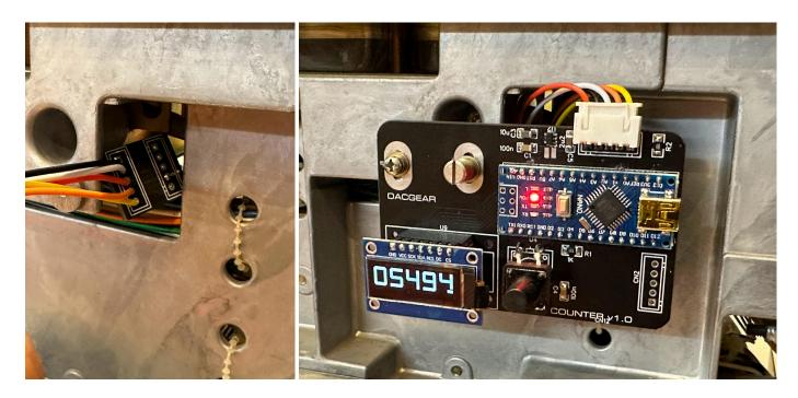
If the display is a bit away from the front panel hole, you can simply pull it out of the socket a few millimetres until It's touching the panel:
