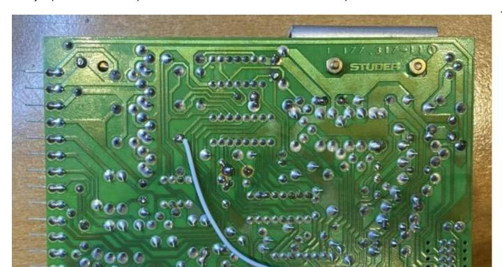
Pull out the pin that sticks out of the connector. This is the pin that is not connected but will be used for direction sensing, and this where the jumper wire connects to underneath. Assemble the connector like in the photo below, making sure that connector pin enters the same position as the original pin that was removed.
