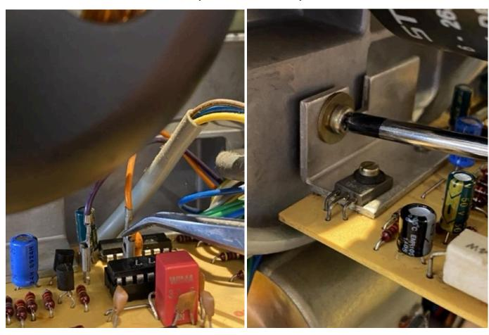
To install the counter tape drive, front and back covers need to be removed first. Then you need to remove the tape control board. Loosen the screw holding the board to the chassis a few turns to the left, but do not remove it completely. The heatsink and the hole board should be able to slide to the left now.
