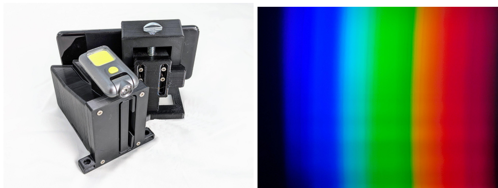
Mobile phone spectrometer design and result with a Samsung Galaxy S10e
