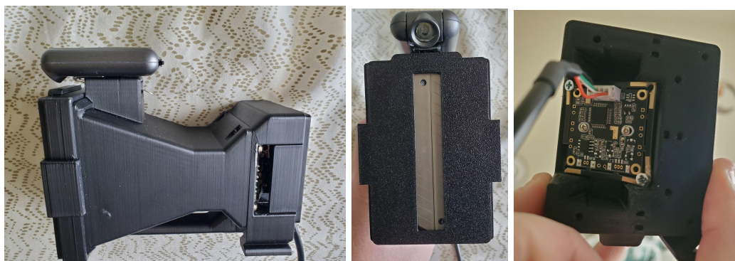
V2 PCB camera design. The cone allows for a 20 degree field of view lens to fill the image with the spectrogram.
