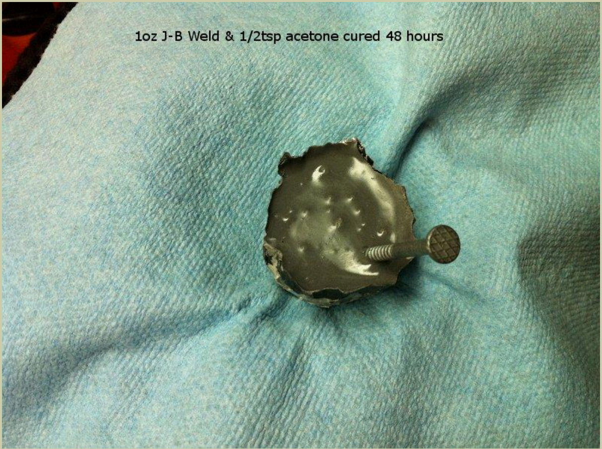
1oz J-B Weld & 1/2tsp acetone after 4 hours at 500F
