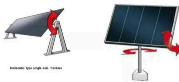
Figure 2-10: Single and Dual Axis Tracker [3]
