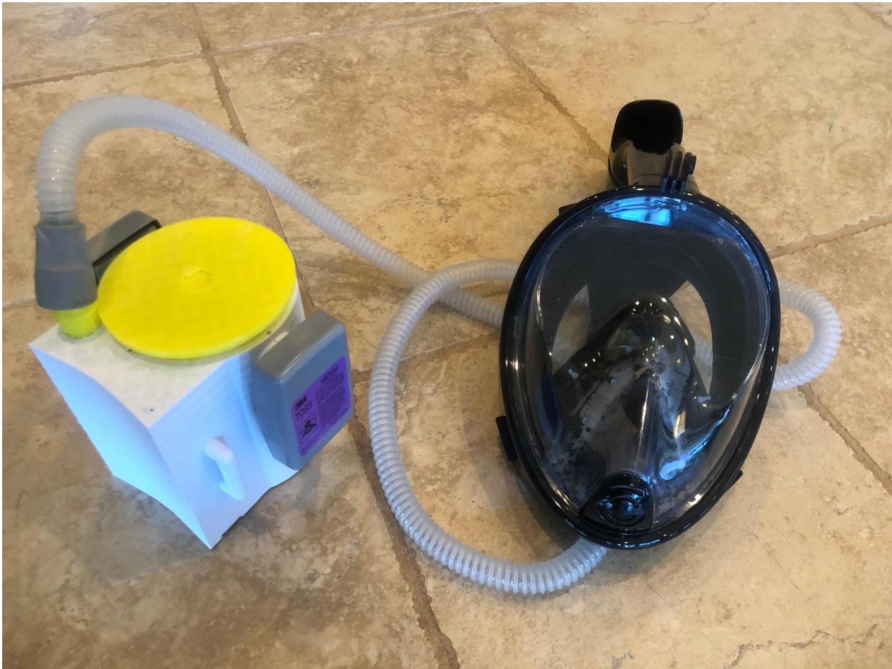
See above: Image of paPURE prototype connected to CPAP hose and snorkel mask. Powered by 4 9V and 4 AA batteries.
