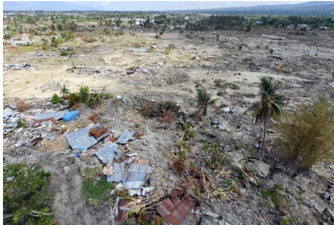
Figure 1: Aerial Photograph of devastation caused by soil liquefaction at Petobo District in Palu, Indonesia (Photo Credit: The Jakarta Post)
