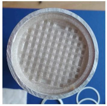
Fill tube with 100 g of silicagel from the one end, then 700 g of zeolite, and then 100 g of silicagel again. Install a second filter from the other end. Add a compression ring.
