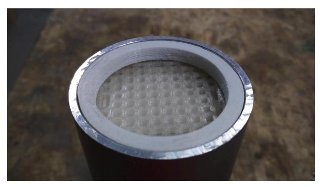
Install sealing rings in caps. Use threaded rods to finish the assembly. Note that zeolite should be compressed inside a bed.
