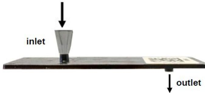
Fig. 2c | Zell Safe™ chip with pipette adapter.
