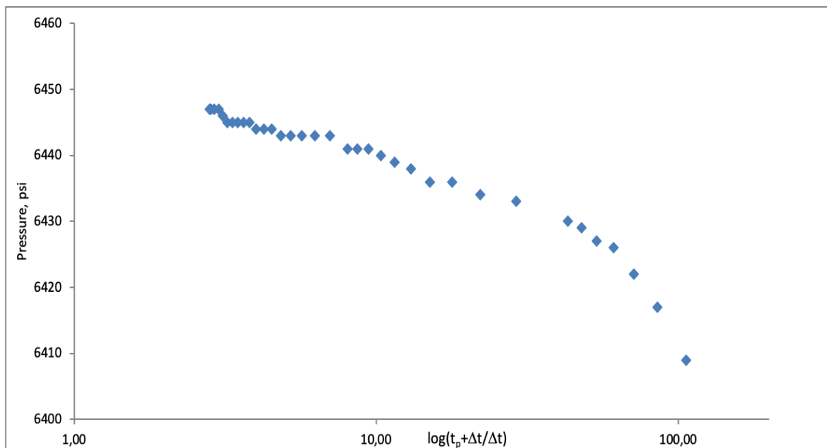
Figure 2.4: Horner Semi-Log Plot (Clemente, 2020).
