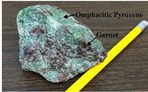
Eclogite facies rock, containing omphacitic pyroxene and garnet
